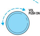
If the volume is set above a certain level and the ignition is turned off, the volume will come back on at a "nominal" listening level when the ignition switch is turned back on. If you wish to maintain your preset volume level, turn the audio system off with the power control before switching off the ignition.
